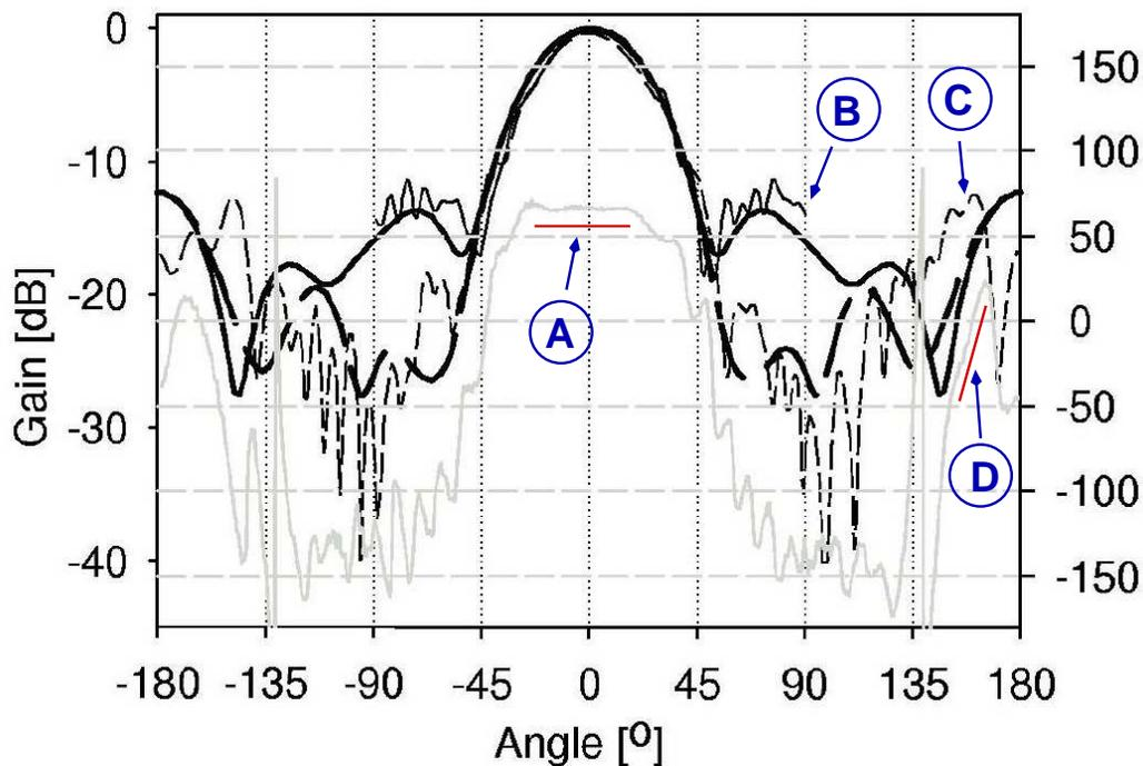
Figure 3: ATA range-measured feed pattern
