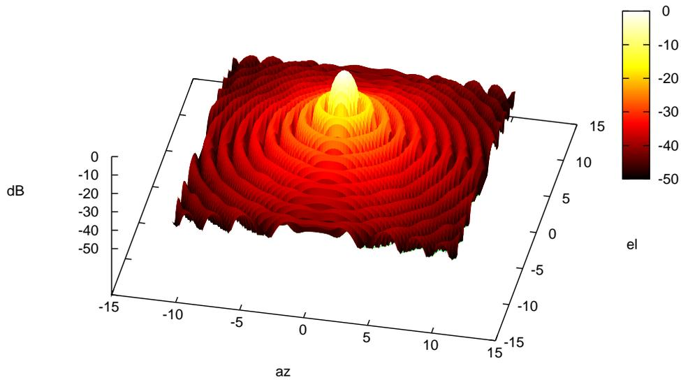
Figure 2: ideal ATA antenna beam pattern (2400 MHz)
